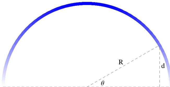
We must also determine the length charge density  $\lambda$  in terms of the variable  $\theta$ . The length charge density is proportional to the distance  $d$  labeled in the plot. Using trigonometry, we have  $d = R \sin \theta$ , so
